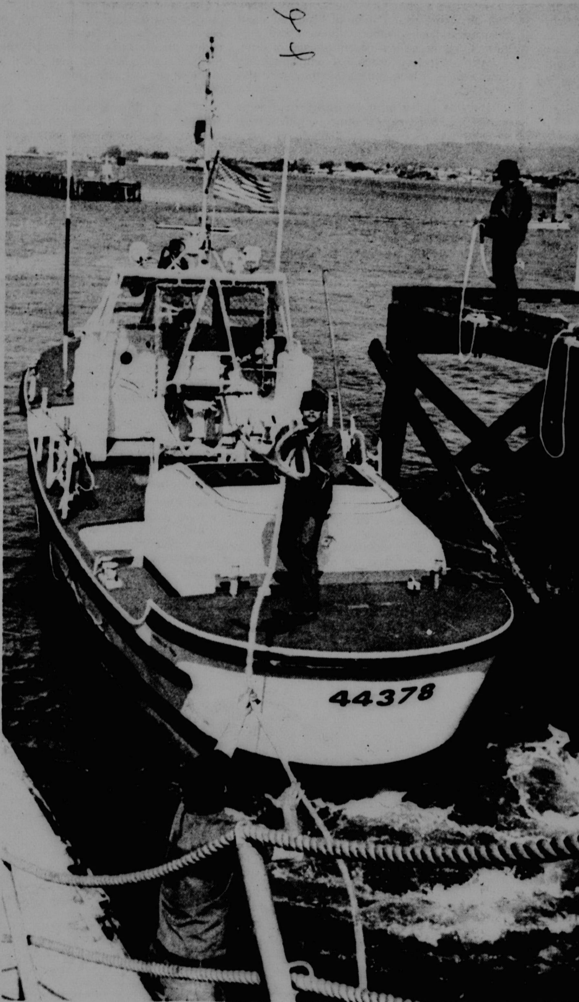
The Coast Guard's 44 foot self-riding motor lifeboat is used primarily for search and rescue situations. It could also be used to board foreign fishing ships in an emergency. The official ship for dealing with foreign trawlers is based in Crescent City.
