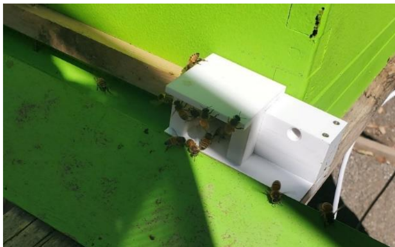
Figure 7. Reader on hive entrance. The reader was screwed into place on the hive entrance with a reducer used to prevent bees from navigating around the reader. A ramp was added to aid in landing at the reader, and to create additional landing space that had been lost with the reader attachment.
