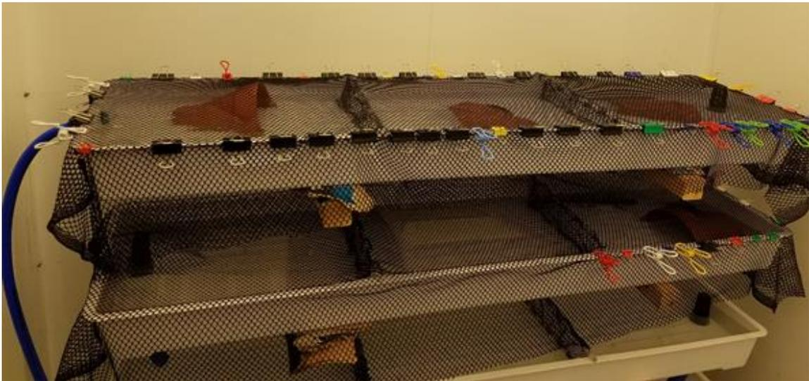
Figure 5: Photograph of the holding tray system for *Dicamptodon tenebrosus*. Each tray was divided into three sections by flow-through partitions. The water was recirculated by a pump kept in a 30-gallon reservoir situated under the trays.
