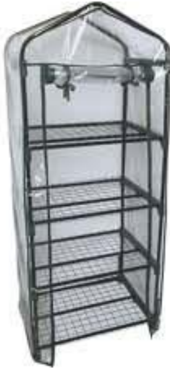
Figure 1. A picture of the Blissun 4 Tier Mini Greenhouse used as a fog chamber in the foliar uptake experiment.
