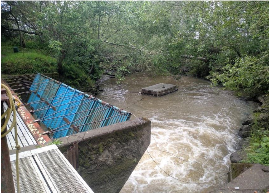
357 358 Figure 4: Modified weir box trap deployed seasonally on the mainstem of Freshwater 359 Creek in Northern Humboldt County, CA.,
