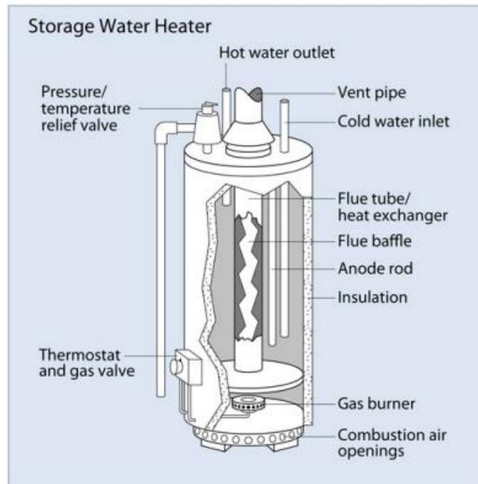
Figure 5. Natural gas storage water heater. (DOE, 2011)
