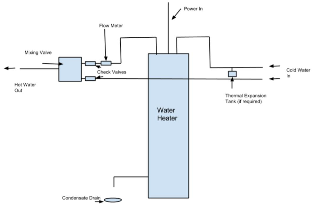
Figure 18. Heat Pump Water Heater with mixing valve and flow meter (ECOFYS, 2014).
