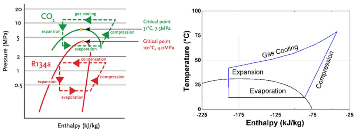
Figure 10. Pressure – Enthalpy (Left) & Temperature – Enthalpy (Right) diagrams for a R744 supercritical cycle where heat is absorbed at constant temperature and subcritical pressure and the heat is rejected at gliding temperature and supercritical pressure (Cibse Journal, 2012).
