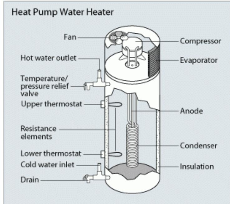
Figure 6. Heat Pump Water Heater (DOE, 2011).
