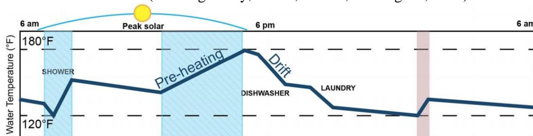
Figure 17. A smart DHW controls when the electric unit in the DHW is engaged to heat water. The water heater preheats the water to a high temperature and then drifts down until the following water draw. (O'Shaughnessy, Cutler, Ardani, & Margolis, 2018)
