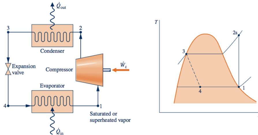
Figure 7. Schematic and Temperature – Entropy diagram for an ideal vapor compression cycle (Moran & Shapiro, 2014).
