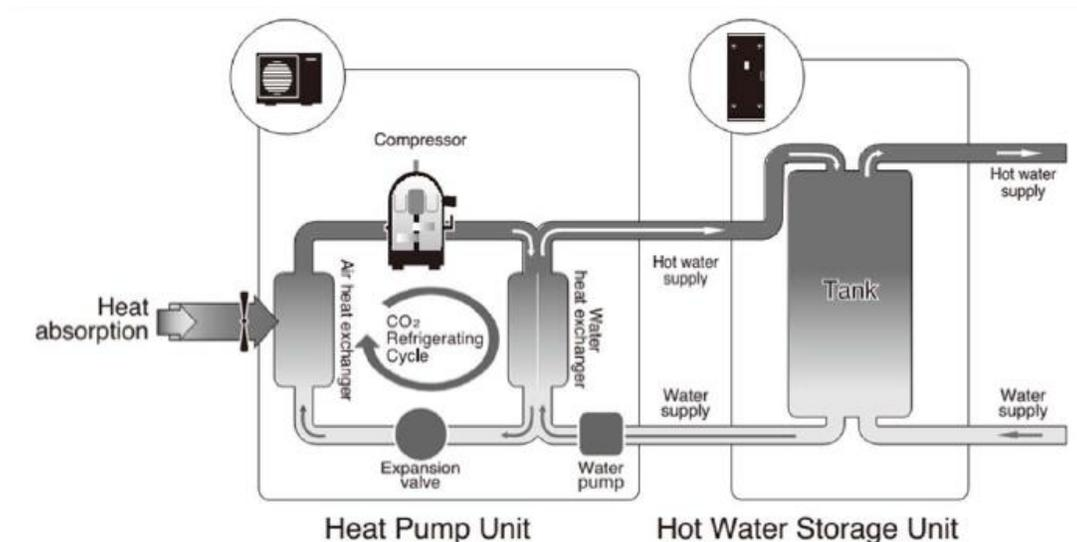
Figure 11. Schematic of Sanden Heat Pump Water Heater Split System. (Sanden, 2018)
