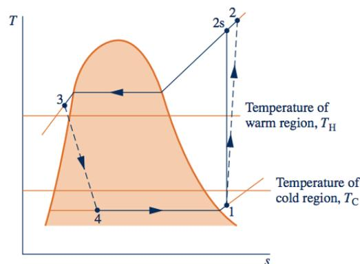
Figure 8. Temperature – Entropy diagram of an actual vapor compression cycle (Moran & Shapiro, 2014).
