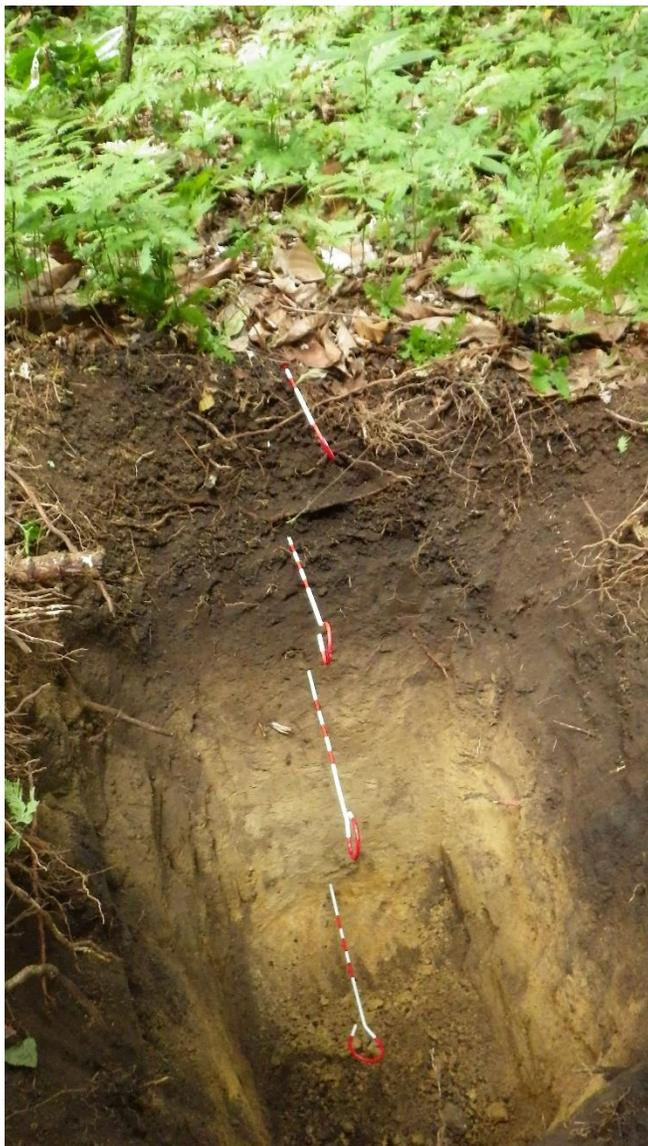
Figure 8. Example of a pedon profile. Horizon designations are identified by red and white pins.
