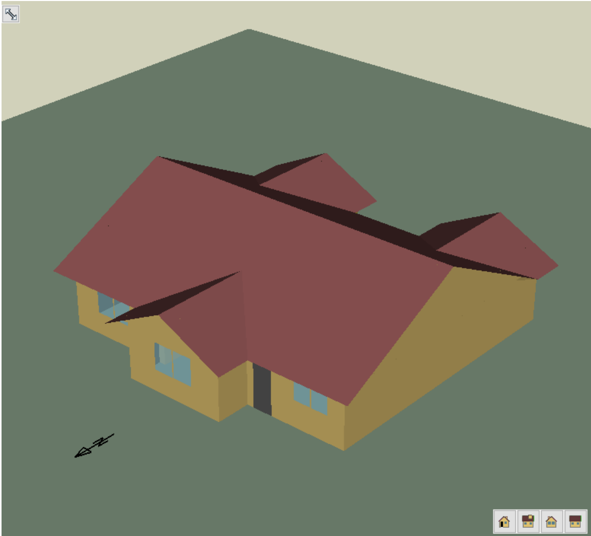
Figure 17: A community services facility for a tiny home village modeled in BEopt 2.8.0.0.
