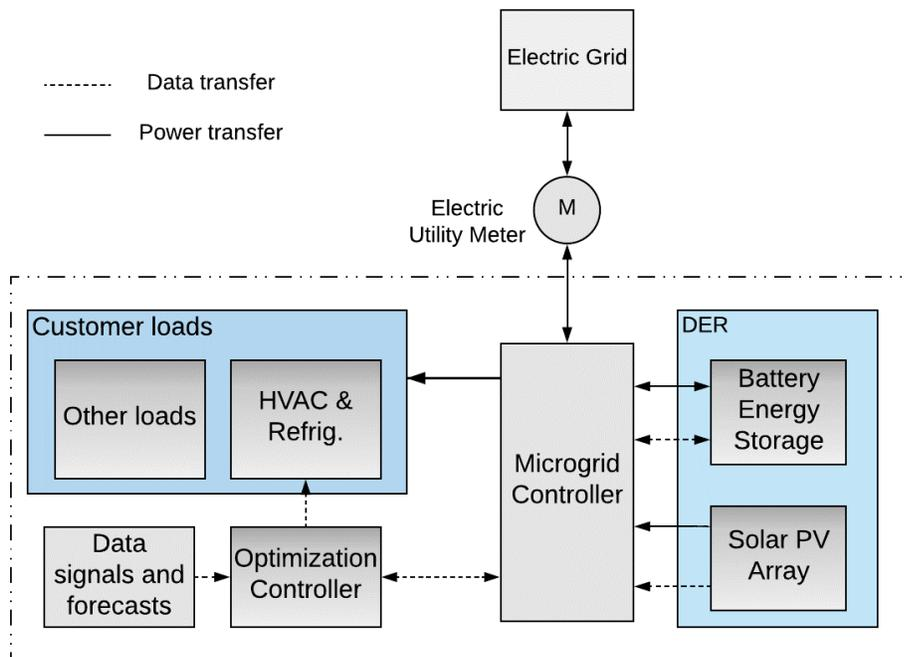
Figure 2. Example of basic MG with solar energy generation, and battery storage as the distributed energy resources, and a MG controller to manage all loads (grid, solar, battery, and customer).
