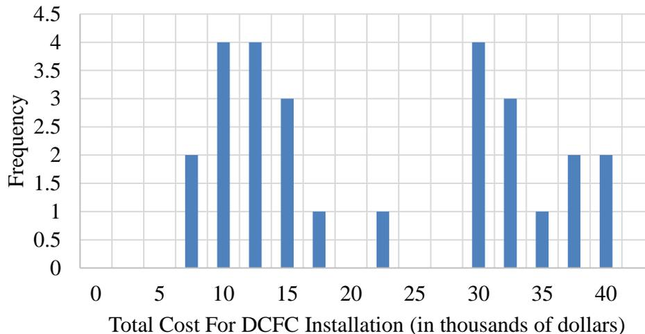
Figure 17. Distribution of DCFC Installation costs for Arizona projects in thousands of dollars. Source: (Idaho National Laboratory 2015).
