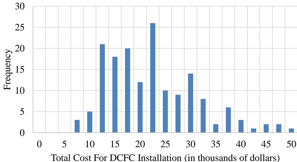
Figure 16. Distribution of installation costs in thousands of dollars for DCFC in 2015. Source (Idaho National Laboratory 2015).
