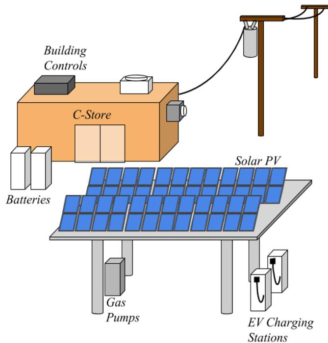
Figure 1. Solar+ microgrid applied to a gas station and convenience store. Adapted from the Schatz Energy Research Center Solar+ Project proposal (Alstone et al. 2016).
