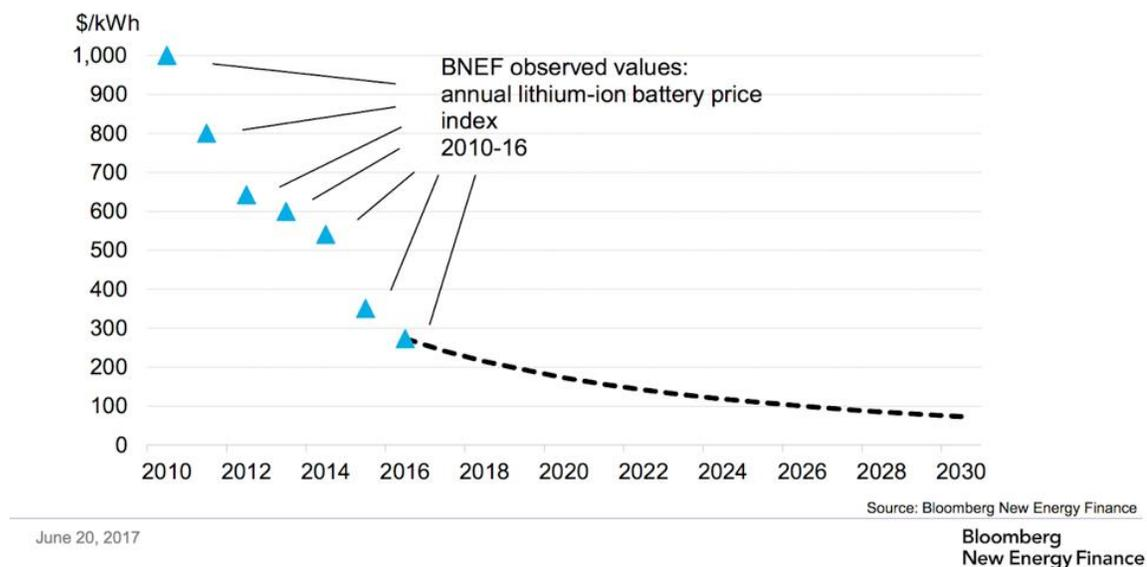
Figure 9. Cost forecast and historical costs for lithium-ion batteries by BNEF. Costs are reported for the years 2010 to 2030. Source: (Curry 2017).
