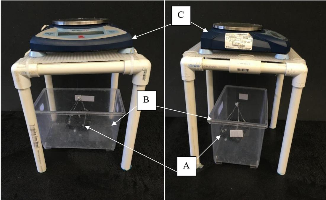
*Figure 2:* Front (Left Panel) and side (Right Panel) view of the hydrostatic suspension measurement apparatus. A mesh basket (A) was submerged in a seawater filled plastic container (B) and attached to a digital scale (C). The mass of submerged mussels can be used to determine the volume of water displaced by the mussel and in turn, the volume of the mussel.
