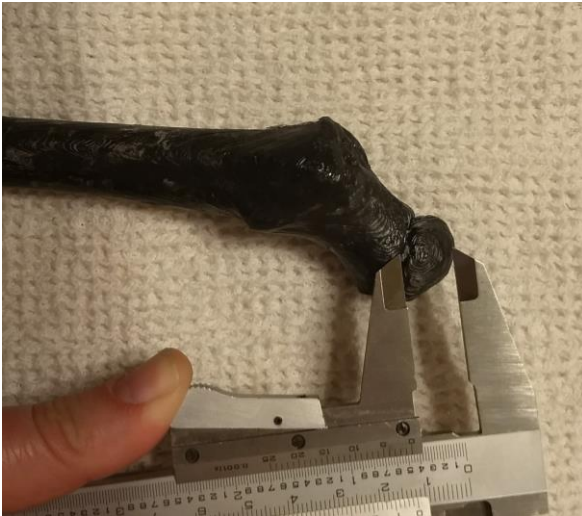
Figure 13: Superoinferior head breadth measurement of 3D printed femur, courtesy of Mercy Children's Hospital, in posterior view
