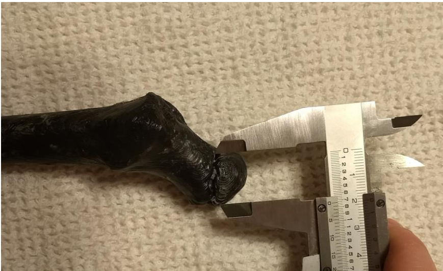
Figure 14: Mediolateral head breadth of 3D printed femur, courtesy of Mercy Children's Hospital, in posterior view
