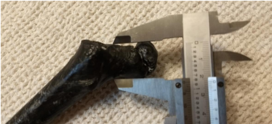
Figure 15: Mediolateral neck breadth measurement of 3D printed femur, courtesy of Mercy Children's Hospital, in posterior view, whereas the measurement is complete due to a missing epiphysis
