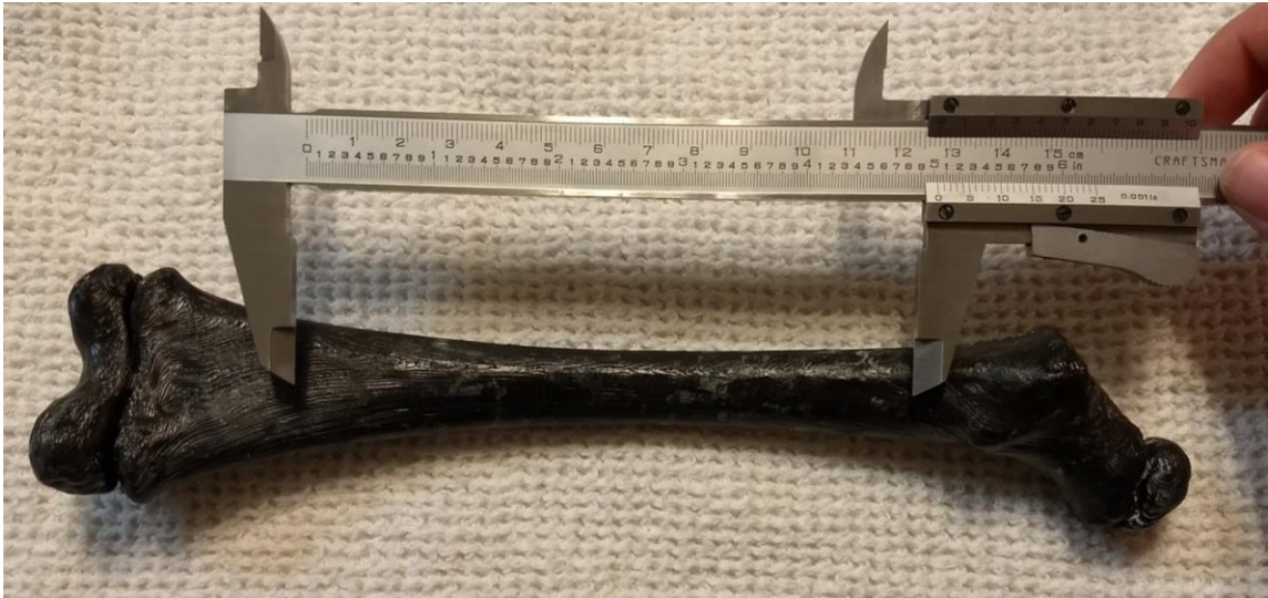
Figure 12: Diaphyseal measurement of 3D printed femur, courtesy Mercy Children's Hospital, in posterior view
