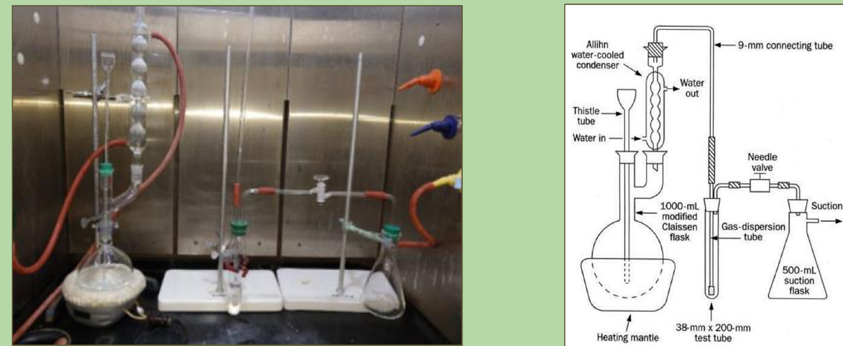
Figure 2: Distillation apparatus for cyanide extraction (left) as compared to specifications in Standard Methods 4500 CN C (right).
