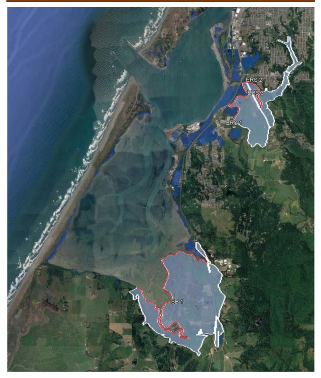
Figure 5. Diked shoreline hydrologic sub-units: Elk River Slough (ERS) and South Bay (SB), diked shoreline reaches (red), and potential MAMW inundation area (blue).
