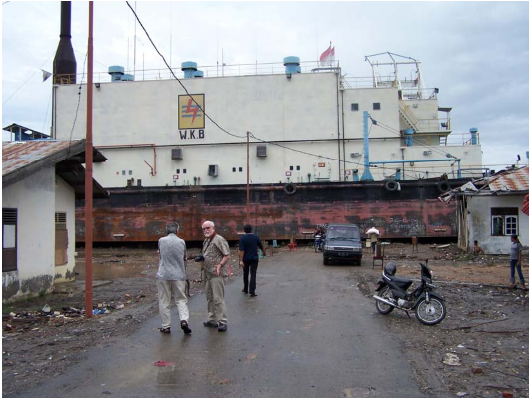
The 10 MW diesel plant was floated 3 km from the coast to its present site by the Dec 26 tsunami. (SN 5/2005)
