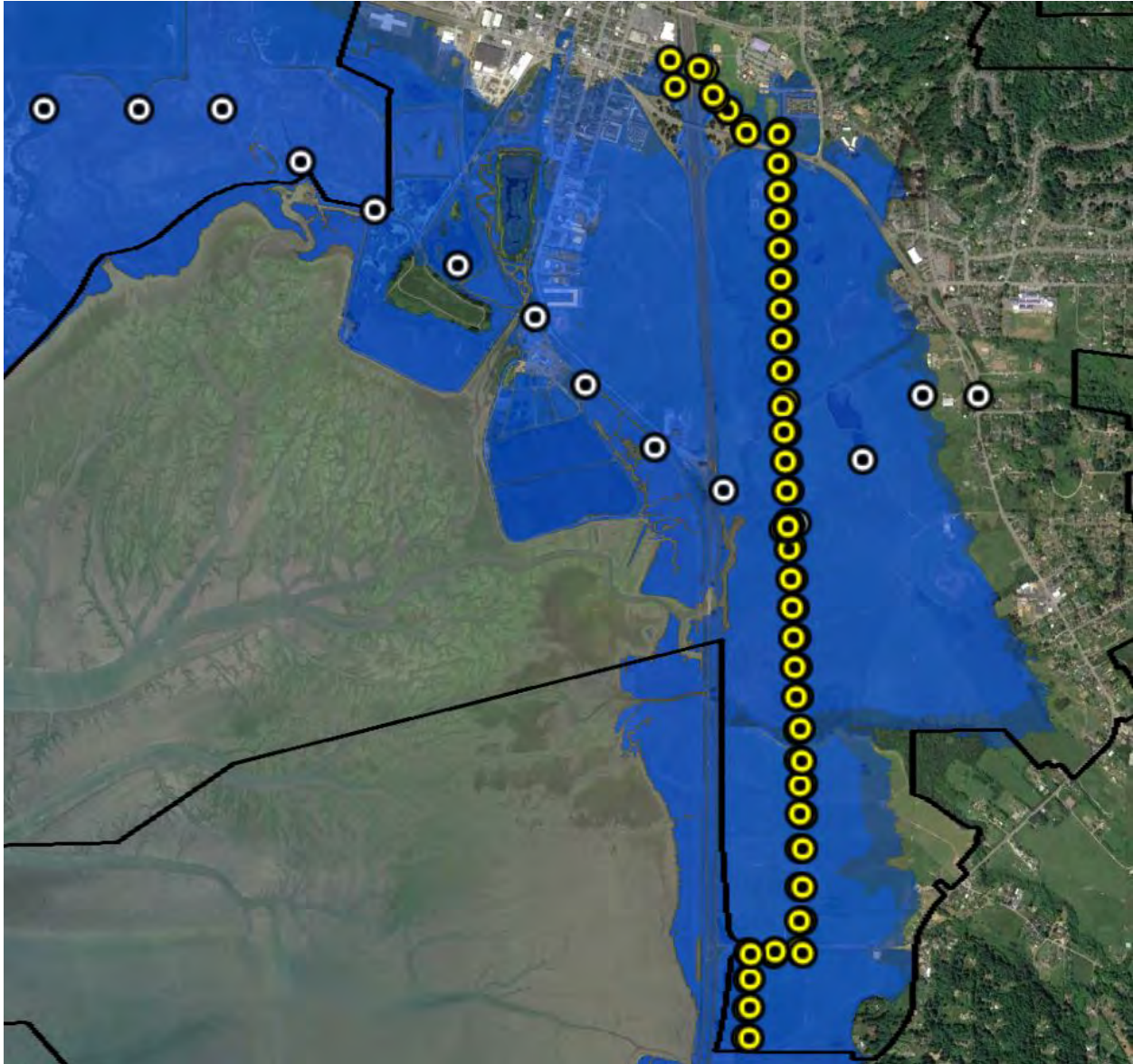
Figure 28. PG&E'S electrical transmission towers (white) and distribution poles (yellow) that could be affected by the tidal inundation from 4.9 ft. (1.5 M) of sea level rise.
