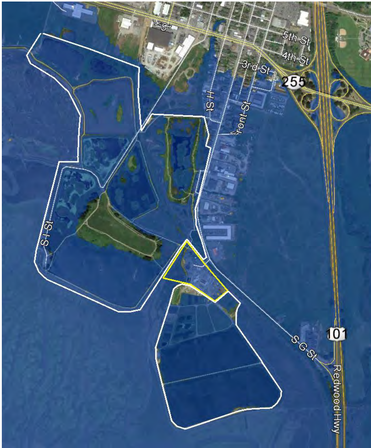
Figure 27. The City's wastewater treatment plant (yellow) and the Arcata Marsh and Wildlife Sanctuary (white) with respect to the tidal inundation area for 3.3 ft. (1.0 M) of sea level rise.
