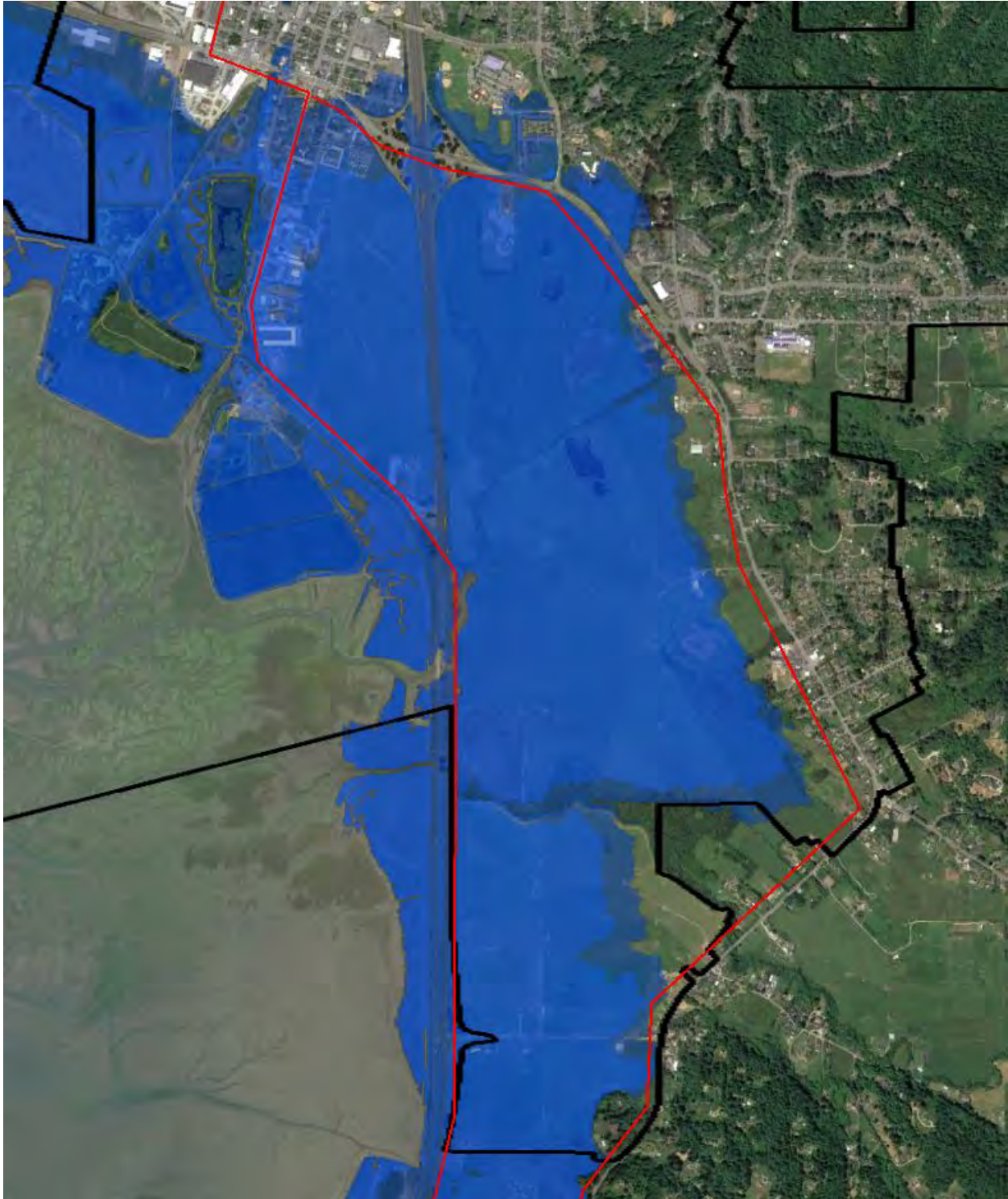
Figure 29. Approximate, location of PG&E natural gas transmission lines (red) in the City of Arcata (black lines) with respect to the 4.9 ft. (1.5 M) sea level rise tidal inundation area.
