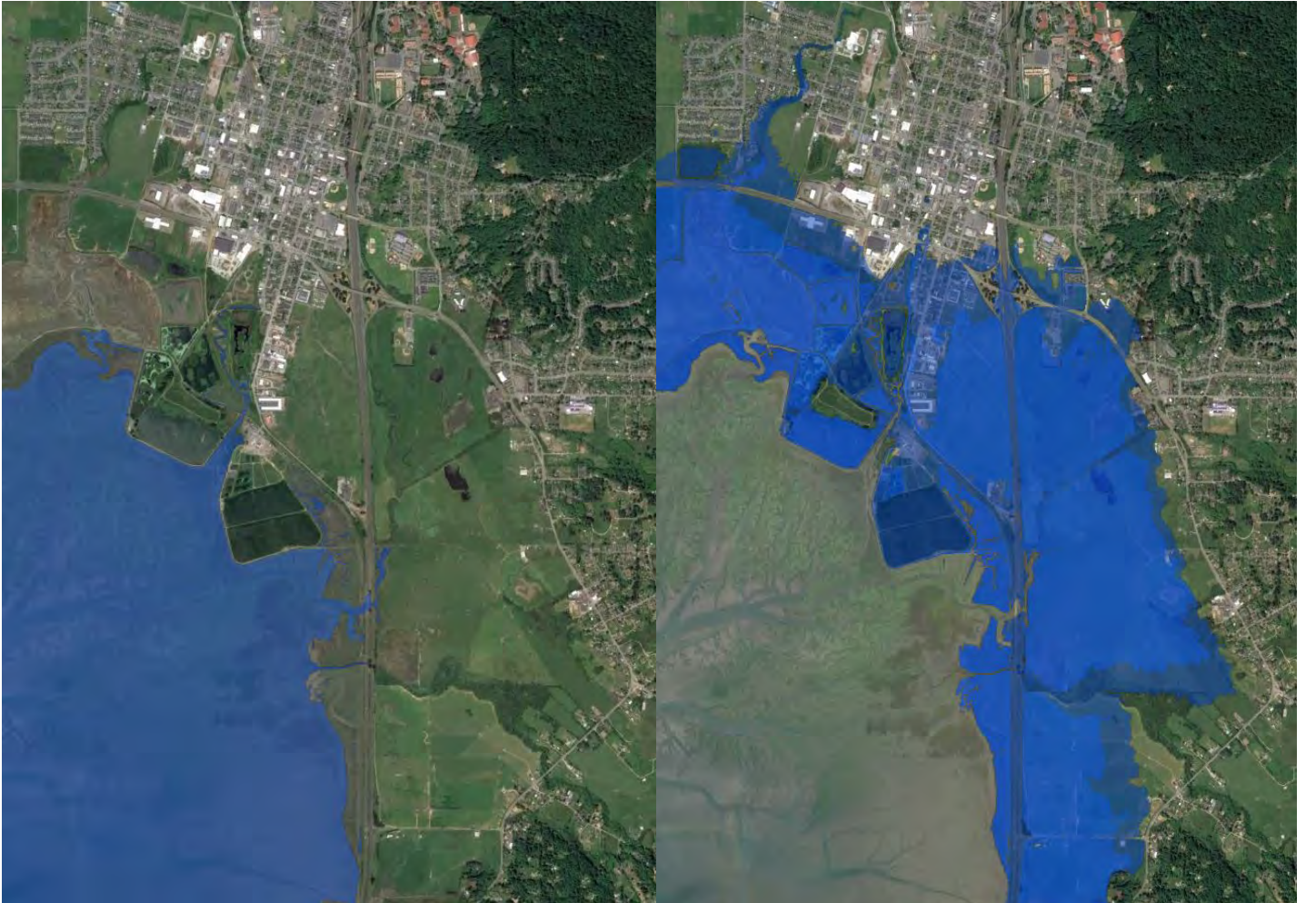
Current Tidal Inundation Areas versus Potential Tidal Inundation Areas (Stillwater) with 4.6 feet (1.5 meters) of Sea Level Rise
