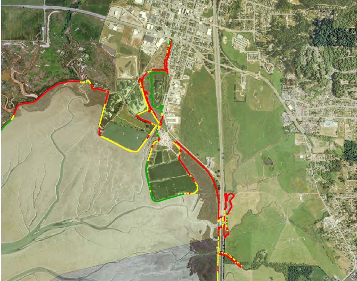
Figure 7. City of Arcata shoreline vulnerability rating: high (red), medium (yellow), and low (green).
