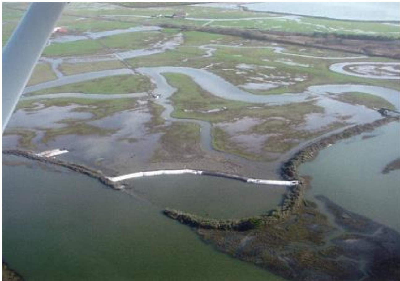
Figure 4. Flooding of pastureland next to Mad River Slough as a result of earthen dikes being overtopped in 2003 ( Times Standard 2003, Laird 2013).
